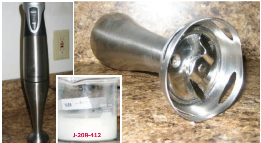
Figure 2: Sheer mixer – laboratory evaluation. Result – 24-hour stability in J-208-412.
